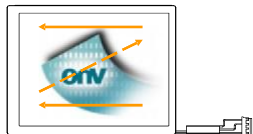
Fig. 2 Reverse scan (Pin4, DPS = High)
