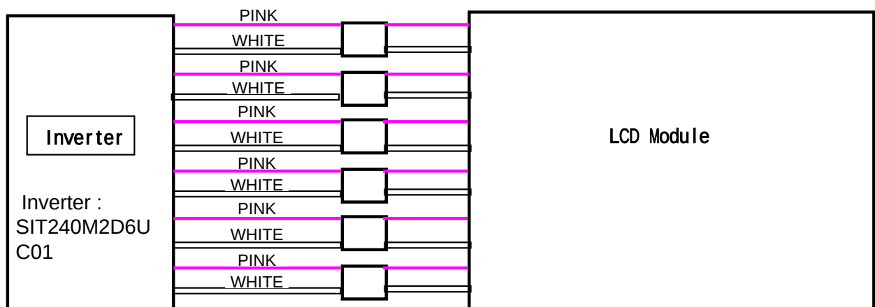
Fig. Measurement point of Lamp Current
