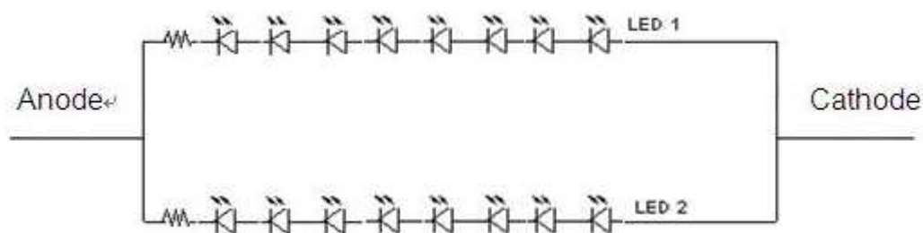
Figure 5 LED Light Bar Structure
